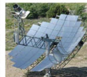
Figure 2.2-2. Dish/Stirling System
